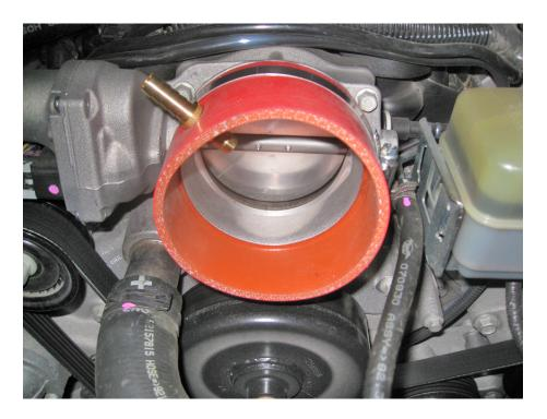
5. Installing the air box (w/air meter attached) into the car.
