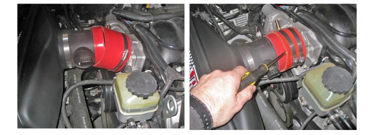
6. Take wiring harness and tuck it under the front as shown in the pic.
