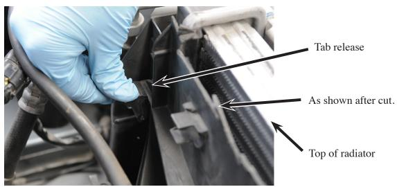
Mark a "HORIZONTAL" line across the backside of the shroud 3/4 inch "BELOW" the top of the radiator line. This removes the small tabs that stick out at the back in one cut.
