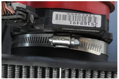
(NOTICE The filter is offset, this allows you to flip the filter by simply rotating it 180 deg. We do this because your throttle body sits at an angle of 8-10deg pointing upward. This just allows you to further compensate for vehicle variation to square everything up in the engine compartment. We like a clean factory racer look, so we have designed in lots of variation.
