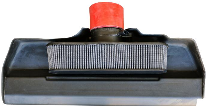
"Notice in the side view the angle cut hose"- this allows you to rotate the filter to the perfect horizontal position, rather than pointing "UP" as your throttle body does.
