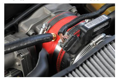
Using supplied PCV hose cut to length and simply press fit hose into place.
