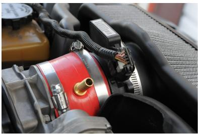
Rotate filter housing so that it sits horizontal not pointed up, this is why we have supplied you with the angle cut hose that is on your throttlebody. (You can cut this hose further if needed)
