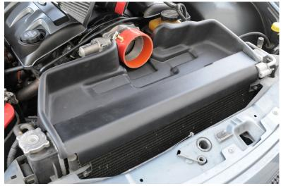
There are no brackets in this kit, the tray is a stressed member that is locked in place by the filter and MAF connection and the hood when it is closed. (Refer to front overview picture if needed)
